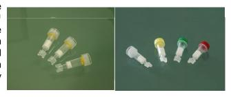
Directions: (p/n: HEM HIL-PSA, HEM HIL-PSA.20, HNS HIL-PSA-M): Cut Off The Outlet Tab with Side-Cut Pliers or a Box Cutter against an elevated support surface. Loosen The Cap when spinning.
