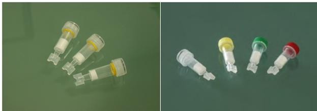
**Directions:** (p/n: **HEM HIL, HEM HIL.20, HNS HIL-M**): Cut Off The Outlet Tab with Side-Cut Pliers or a Box Cutter against an elevated support surface. Loosen The Cap when spinning.
