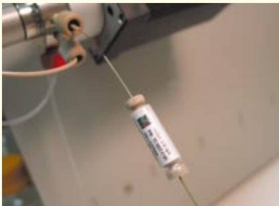
The Capellini column's robust, inert, and symmetrical design permits column backflushing.
