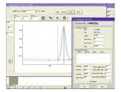
control approval. This testing protocol involves a highly accurate statistical moments determination of the column's performance characteristics. These sensitive peak shape and column efficiency measurements can only be made by computerized data logging methods. The raw digital chromatogram for every column we have manufactured since March 1994 is retrievable from our archives.
