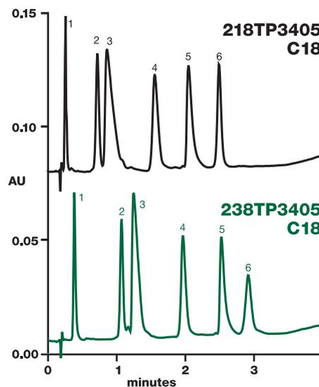
Figure 3. Comparison of peptide separation on two 3 $\mu$ m 300Å reversed-phase columns. Flow rate: 4.0 mL/min. Columns: Same as Figure 2. Mobile phase: A = 15% acetonitrile (v/v) in water with 0.1% TFA (w/v). B = 25% acetonitrile (v/v) in water with 0.1% TFA (w/v). Gradient: 0% to 100% B in 3 minutes. Detection: 215nm. Sample: Peptide mixture. Peaks: (1) neurotensin fragment 1-8, (2) oxytocin, (3) neurotensin fragment 8-13, (4) angiotensin II, (5) neurotensin, and (6) angiotensin I.
