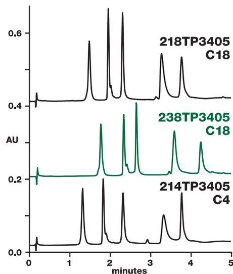
Figure 2. Comparison of protein separation on three 3 $\mu$ m 300Å reversed-phase columns. Flow rate: 4.0 mL/min. Columns: Vydac 218TP3405 "polymeric" C18, 238TP3405 "monomeric" C18, and 214TP3405 C4, all 4.6mmID x 50mmL. Conditions: As described for Figure 1. Sample: Standard protein mixture. Peak order: Same as Figure 1.
