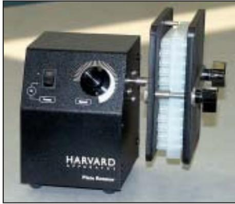
A Plate Rotator with variable rotation rates is available for use with Harvard/AmiKa's Equilibrium Dialyzer-96™. The Rotator speeds up the equilibrium dialysis process by keeping the sample in constant motion ensuring higher reproducibility of results.
