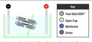
Configuration B: Selective Electro-Filtration/Concentration/Separation Based on Different Charges on Biomolecules
