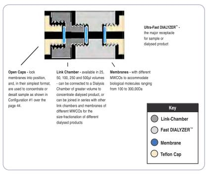
As shown above, multiple link chambers can be joined together with membranes of different MWCOs placed between them for highly selective electro-filtration and separation.
