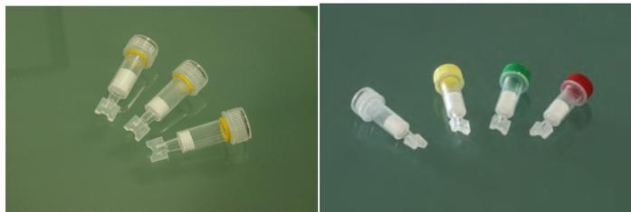
**Directions:** (p/n: **HMM HIL-WCX, HMM HIL-WCX.20, HNS HIL-WCX-L**): Cut Off The Outlet Tab with Side-Cut Pliers or a Box Cutter against an elevated support surface. Loosen The Cap when spinning.
