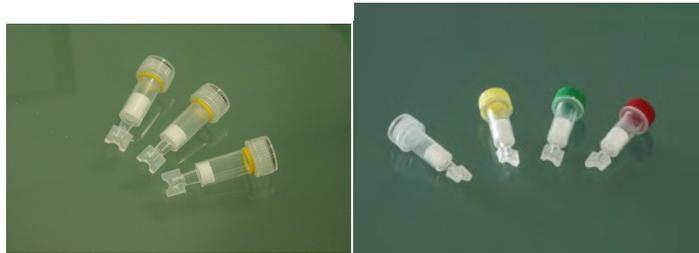
**Directions:** (p/n: **HMM HIL-WCX, HMM HIL-WCX.20, HNS HIL-WCX-L**): Cut Off The Outlet Tab with Side-Cut Pliers or a Box Cutter against an elevated support surface. Loosen The Cap when spinning.
