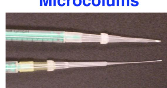
Figure 2: Microcolumn in GELoader
