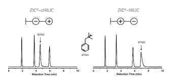
**ZIC®-cHILIC** is designed for excellent HPLC and LC-MS analysis of polar hydrophilic compounds. This new zwitterionic stationary phase with phosphorylcholine functional group provides you with complementary selectivity for easier method development for substances that have been difficult to separate by previous types of HPLC columns operated in reversed-phase or HILIC mode.
