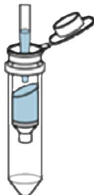
2. Centrifuge the column with the collection tube at 800 x g for 2 minutes to collect the sample. Discard the column after use. Now the sample is ready for downstream analysis.
